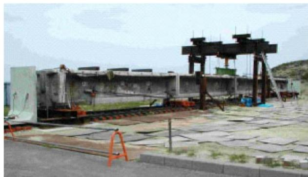
写真-1 撤去桁の載荷試験<sup>1)</sup>
